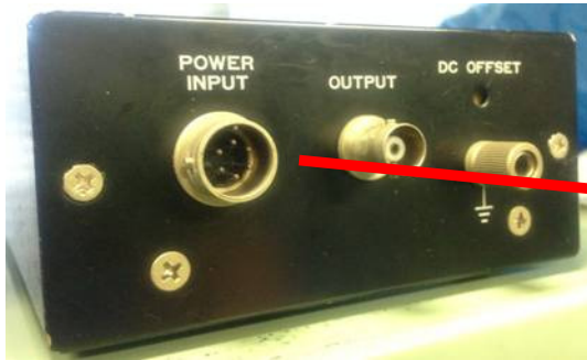
Power Input Connection in Rear Panel of LI-75A
