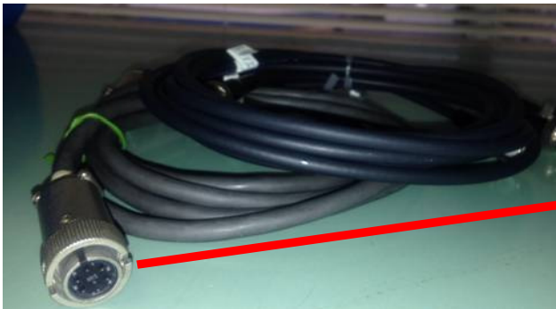
Power cable Connection in Power cable of LI-75A
