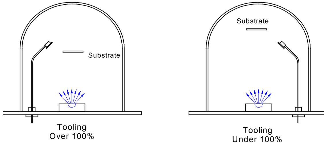
**xTooling** is set in the System Menu. It adjusts the tooling for each individual sensor before it is averaged. xTooling for a sensor applies to all films. If the individual sensor xToolings are set properly, a sensor failure will not cause a jump in the average Rate and Thickness reading.
