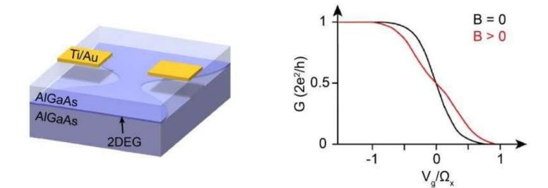
Quantum point contact structure (left) in which an applied voltage constricts electron movement to one dimension, with conductance (right) showing effect of applied magnetic field (red). Credit: UNSW
