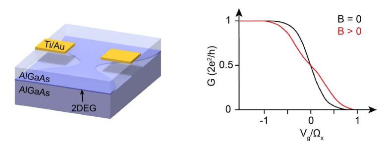
A quantum point contact structure (left) in which the applied voltage limits the movement of electrons to one dimension and the conductance (right) shows the effect of the applied magnetic field (red). Credit: UNSW
