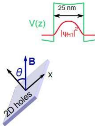
Upper right GaAs hole quantum well used in the study. Lower left: device is tilted at an angle to applied magnetic field.
