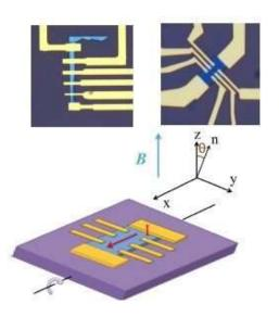
2-D WTe2 samples (upper) and experimental schematic (lower) diagram of angle-dependent measurement configuration. Credit: FLEET
