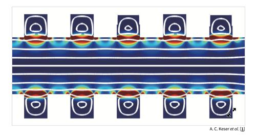
**Thicker than honey.** This image from a simulation shows streamlines (white) of electrons flowing as a viscous fluid. The loops show that the fluid forms eddies in the crenelles. Colors indicate the power dissipation at each location, from zero (dark ... **Show more**
