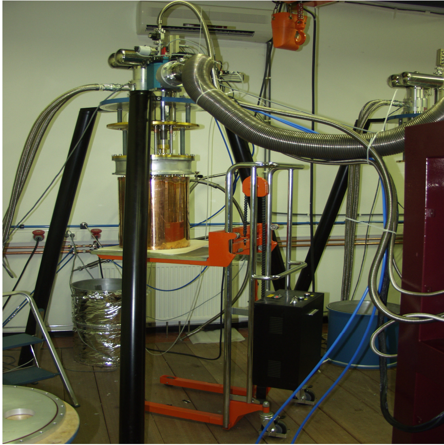
Figure 11 It is recommended to use a stacker to mount and dismount the radiation shields.
