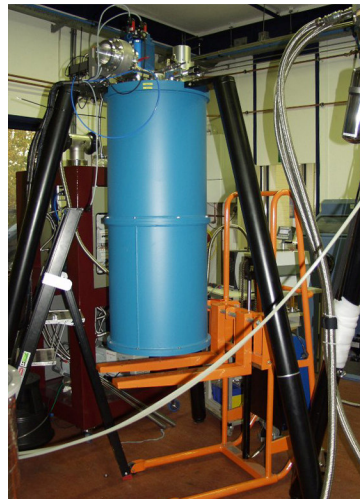
Figure 3 It is recommended to use a stacker to lift the cryostat.
