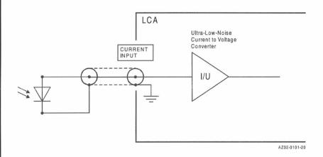
Photo Detector Biasing in Photoconductive Mode: Use for Fast Applications and if More Dark Current is Tolerable. Bias Voltage Decreases Detector Capacitance.
