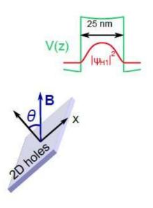
Upper right GaAs hole quantum well used in the study. Lower left: device is tilted at an angle to applied magnetic field. Credit: FLEET
